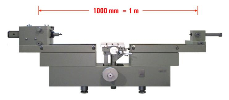
The DMS 680 can be equipped with a special extension to increase its capacity up to 1000 mm external.
